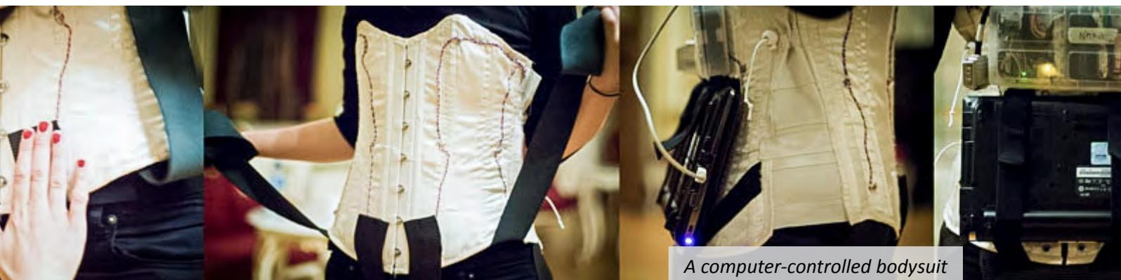
The bodysuit is a stand-alone application based on mini-pc's in combination with custom built Arduino controller-board. It is an open-source project working with the development of haptic and tactile storytelling.
